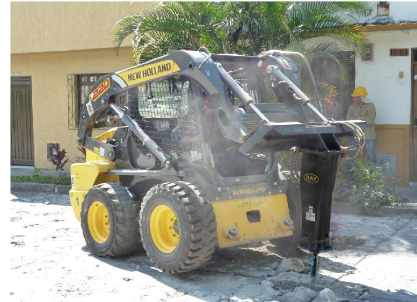
Skid steer loader : NEW HOLLAND L220 Hydraulic breaker: RHB68 Box silence type Country: Australia
